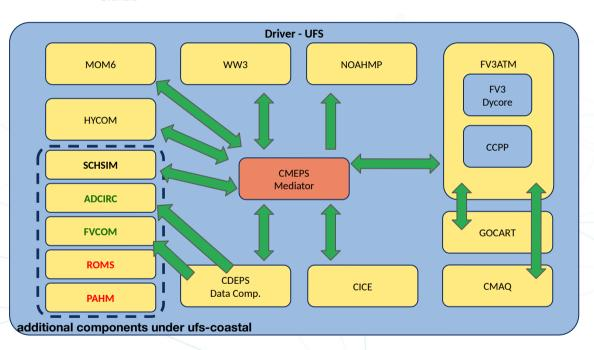
ADCIRC and FVCOM model components are under development ROMS and PAHM are future model component capabilities
